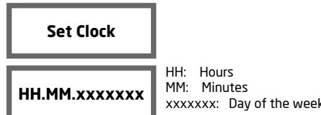
Press the UP/DOWN buttons to change the **HOURS** and press **OK** to confirm and move on to the **MINUTES** and the day of the week. After confirming the day of the week, it will automatically go into the weekly ON/OFF programming mode.
