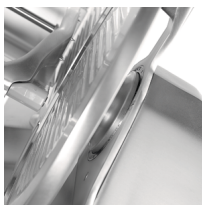
Enclosed and sealed belt pulley standard
